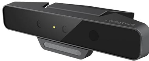
**Figure 3:** Intel Realsense SR300 RGB-D Camera.
